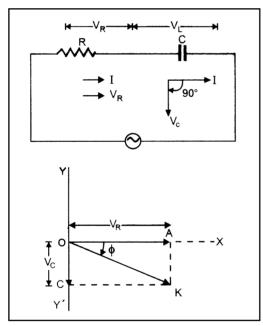
Figure represents phasor diagram of RC circuit. We find that in RC circuit, voltage lags behind the current by a phase angle  $\phi$ , where
