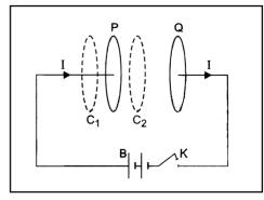
Due to battery B, let the conduction current I be flowing through the lead wires at any instant, but there is no conduction current across the capacitor gap, as no charge is transported across this gap.
