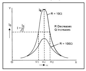
The Q factor of series resonant circuit is defined as the ratio of the voltage developed across the inductance or capacitance at resonance to the impressed voltage, which is the voltage applied across R.
