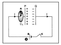
Now, we consider a different surface, i.e., a tiffin box shaped surface without lid with its circular rim, which has the same boundary as that of loop  $C_1$ . The box does not touch to the connecting wire and plate P of capacitor. The flat circular bottom S of the tiffin box lies in between the capacitor plates. Figure (b). No conduction current is passing through the tiffin box surface S, therefore I = 0. On applying Ampere's circuital law to loop  $C_1$  of this tiffin box surface, we have
