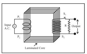
For an ideal transformer, we assume that the resistances of the primary and secondary windings are negligible.
