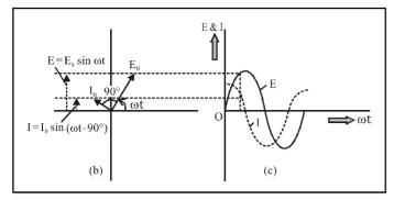
Comparing (3) with Ohm's law equation, viz current = voltage/resistance, we find that  $(1/\omega \text{ C})$  represents effective resistance offered by the capacitor. This is called capacitative reactance and is denoted by  $X_{C}$ .
