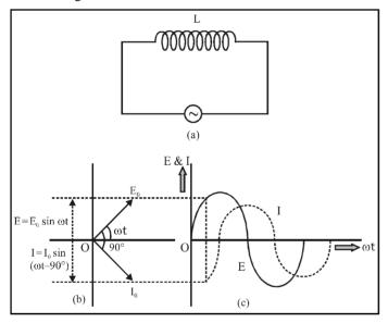
Figure (b) represents the vector diagram or the phasor diagram of a.c. circuit containing L only. The vector representing  $\vec{E}_0$  makes an angle ( $\omega$ t) with OX. As current lags behing the e.m.f. by 90°, therefore, phasor representing  $\vec{I}_0$  is turned clockwise through 90° from the direction of
